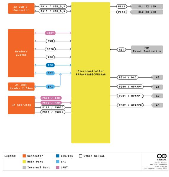
Arduino R4 Minima Block Diagram
