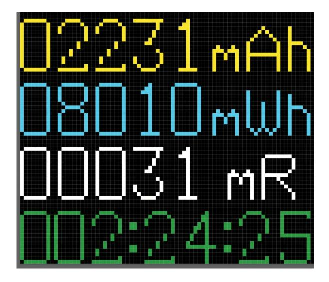
One click all channel discharge capacity measurement: Press and hold the "通道/CHN" button for 3 seconds, and the full channel will run in the "discharge" mode according to the preset stop voltage of 3.0V.。
