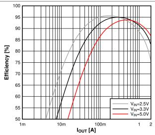
Figure 9-9. 1.8-V Output Efficiency (TPS62A02)
