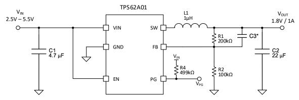
Figure 9-1. TPS62A01 Typical Application Circuit
