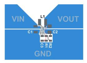
Figure 11-1. TPS62A0x PCB Layout Recommendation
