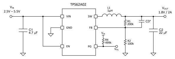
Figure 9-2. TPS62A02 Typical Application Circuit
