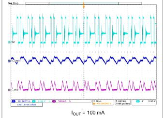
Figure 9-12. Power Save Mode Operation
