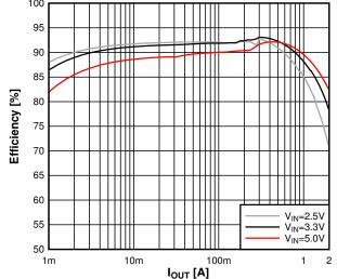
Figure 9-7. 0.6-V Output Efficiency (TPS62A02)
