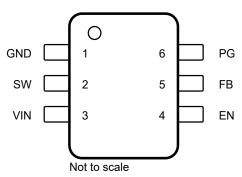
Figure 6-1. 6-Pin DRL SOT-563 Package (Top View)
