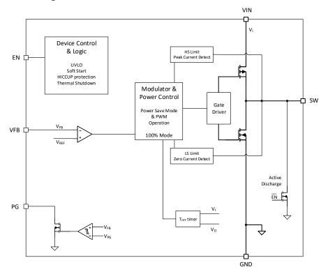
Figure 8-1. Functional Block Diagram
