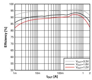
Efficiency vs Output Current at 5 VIN
