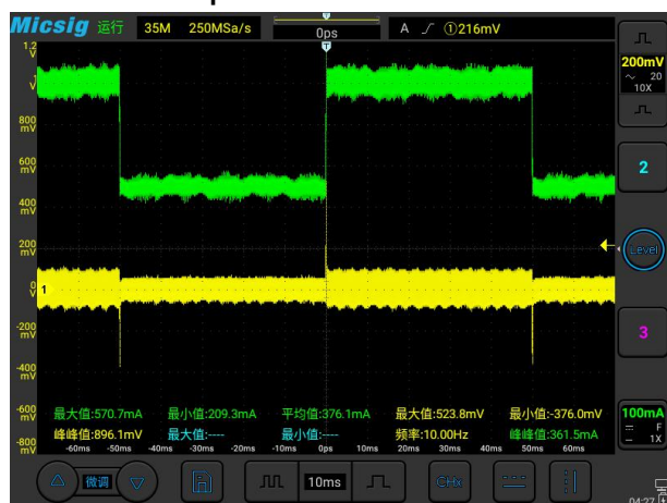
Transient Response VIN=52V, Io=50%~100%~50%
