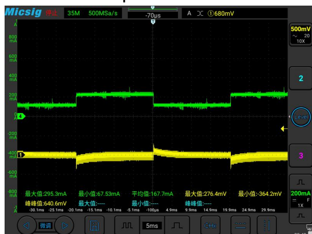
Transient Response V_{IN}=52V , I_o=50\% \sim 100\% \sim 50\%
