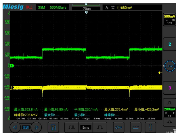
Transient Response VIN=52V, Io=50%~100%~50%
