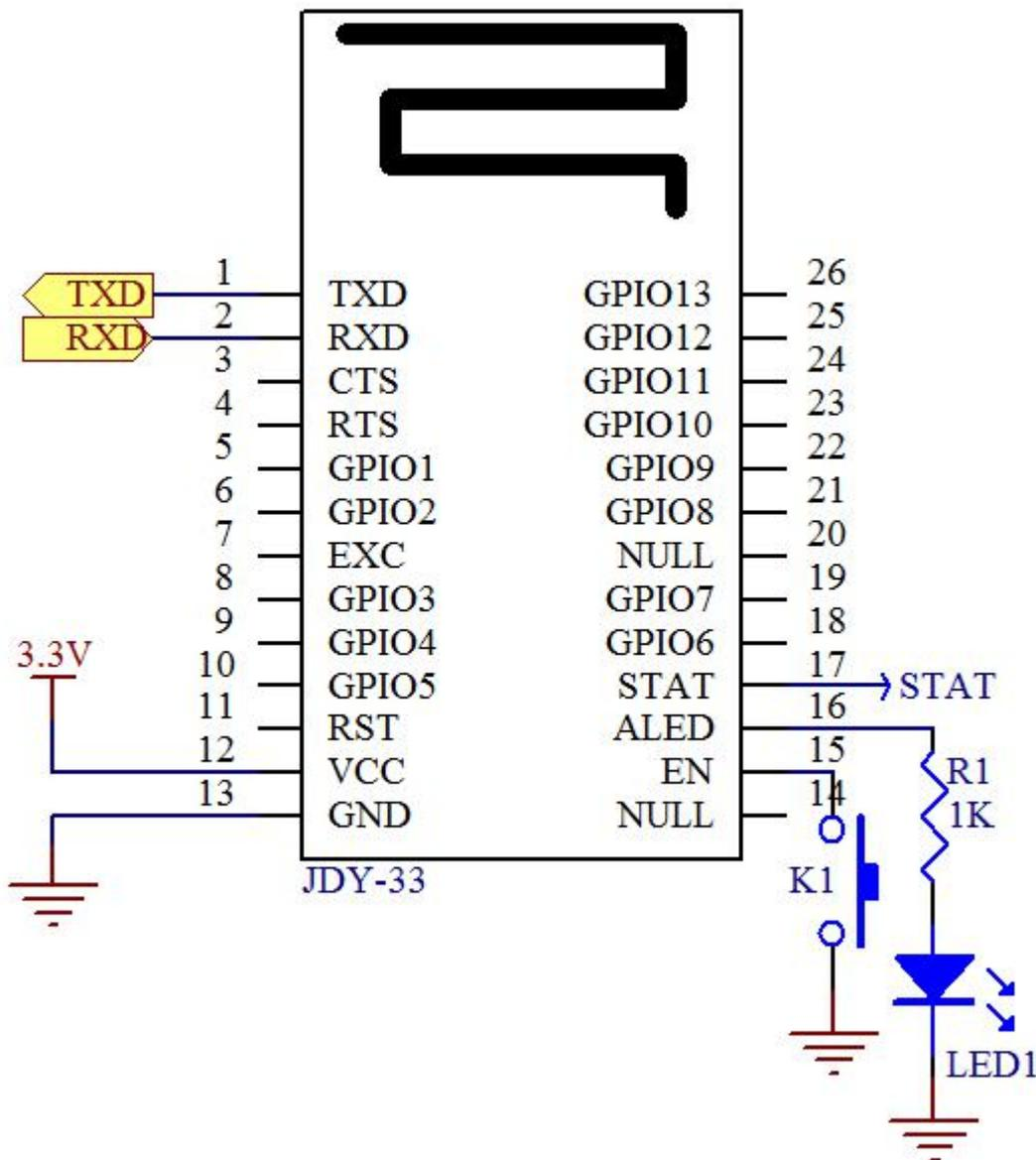
JDY-33 applications only need to connect VCC, GND, RXD and TXD pins. The connection state requires a disconnect, send AT+DISC\r\n. Send AT+SLEEP\r\n for deep SLEEP in unconnected state. Deep sleep can be awakened by the falling edge of EN pin, or by sending data through serial port. It is generally recommended to use serial port to send AT+VERSION\r\n instruction to wake up.
