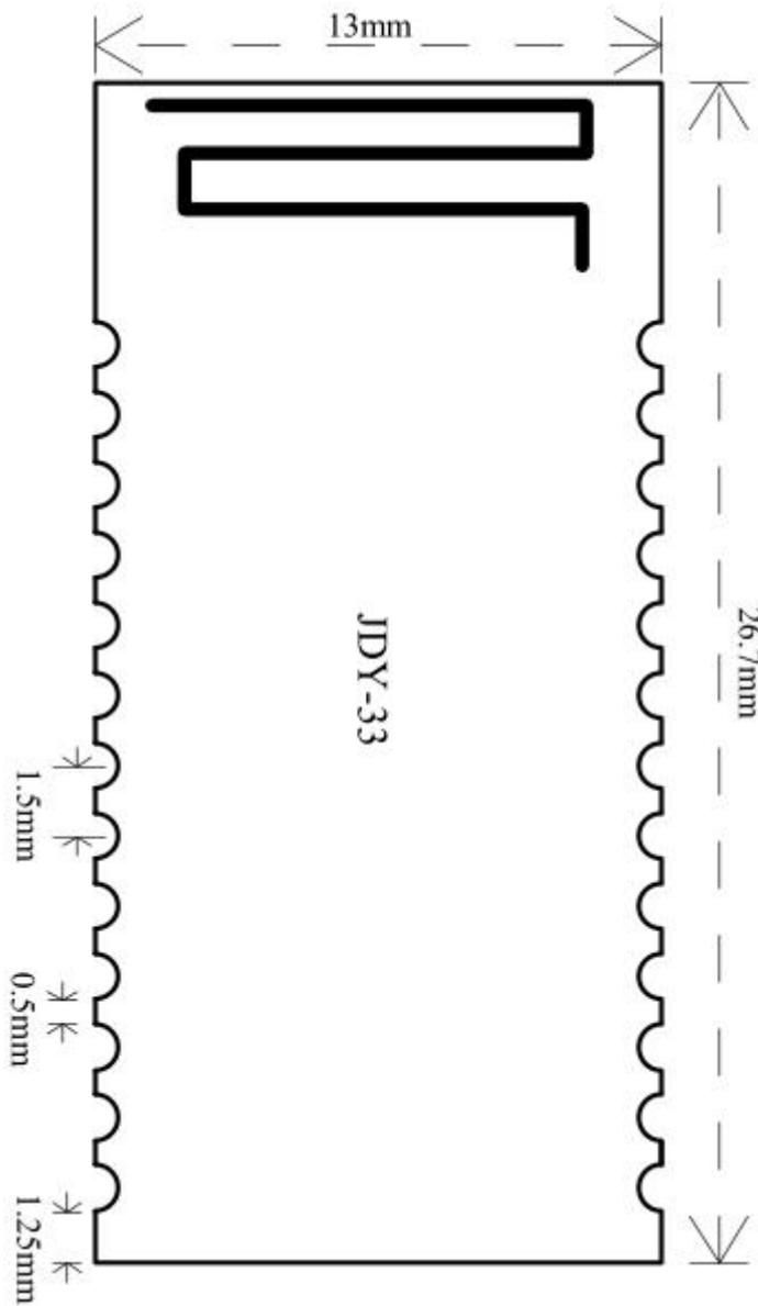
PCB package is fully compatible with JDY-30, JDY-31, JDY-09, JDY-32
