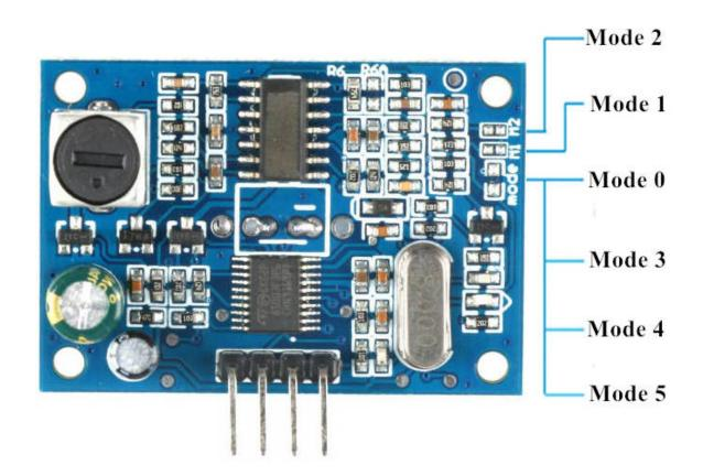
Mode 0: Mode floating = trigger pulse width output (factory default mode)
