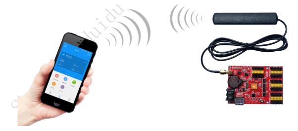
**Scheme two:** Connect to the control card via router, mobile phones are connected via this wireless router.
