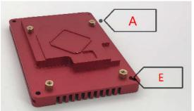
Put the heat conductive paste in the designated CPU space in the middle of the the heatsink. (less is more – please only place a small drip in the center!)
