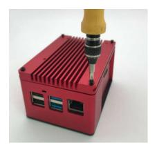
the heatsink. Use the silicon feet and stick them on the outer sides of the heatsink.
