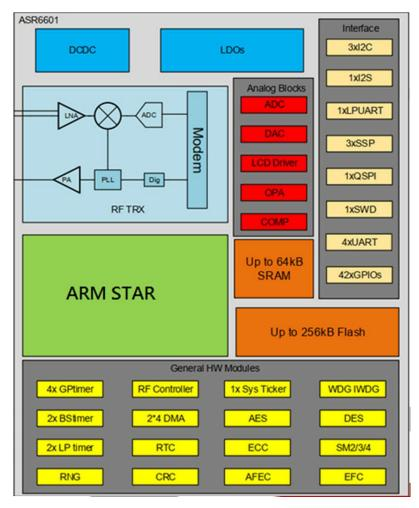
Figure 1 Main chip architecture diagram
