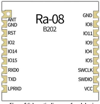
Figure 5 Schematic diagram of module pins
