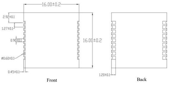
Figure 4 Module size diagram
