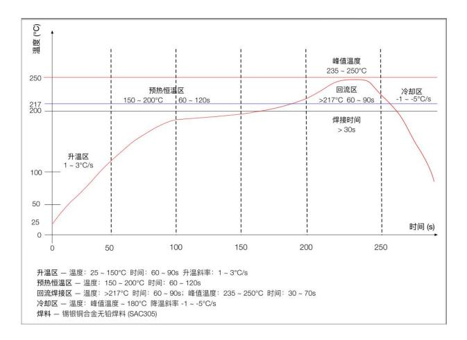
Figure 11 Flow welding diagram
